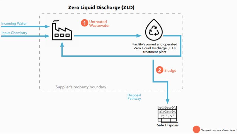
Figure 2d: Schematic illustration of the Wastewater Discharge Types and Sample Locations. Sampling locations: Untreated Wastewater, Sludge.
