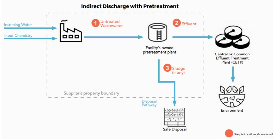
Figure 2b: Schematic illustration of the Sample Locations for an Indirect Discharge with pretreatment Supplier. Sampling locations: Untreated Wastewater, Effluent, Sludge.
